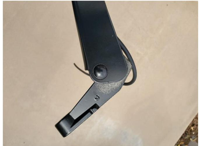
This may take a bit of work or an extra pair of hands because the spring is very strong and this step is required to enable pushing the wiper arm straight over the wiper motor post. The post is cone shaped with grooves while the arm although having a cone shaped hole is not grooved.
