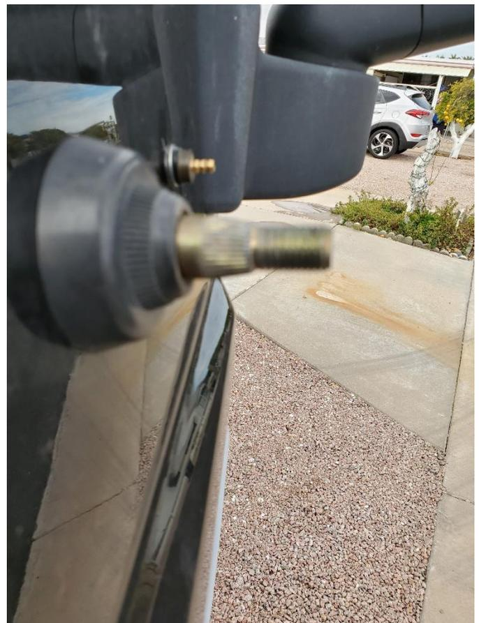
Proper alignment critical. If you are as lucky as I was there are alignment marks on the end of the wiper motor post. Push the arm on the post, add the washer, then slightly snug the bolt just enough to keep the wiper arm in place. Fold the wiper to the glass to check positioning to make sure that when moving the wipers will not hit each other.
